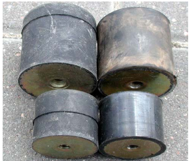
Rubber joint safe(left), and unsafe (right)
